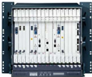
Figure 1. Cisco ONS 15454 ANSI/SONET System
